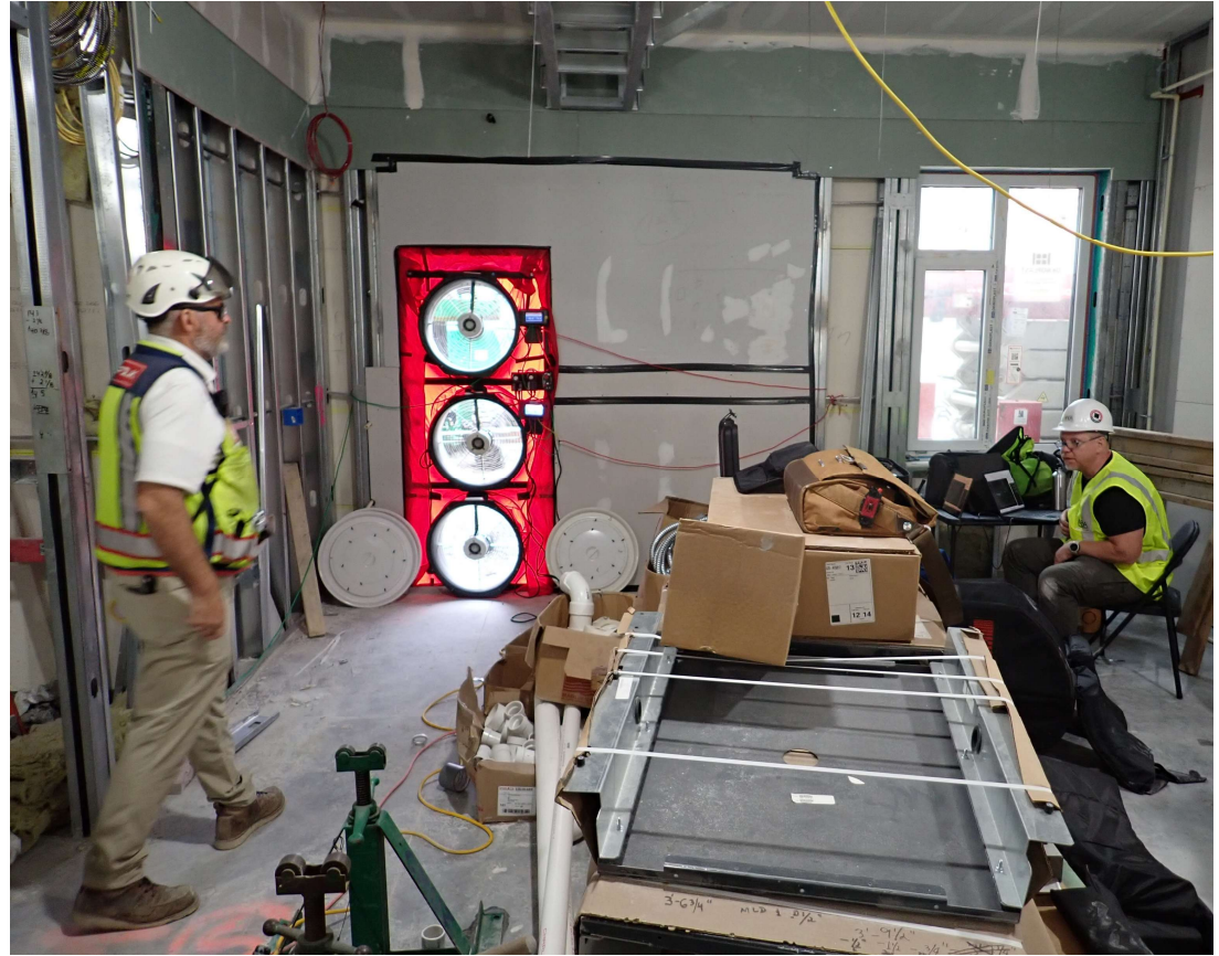
Whole Building Airtightness Testing
