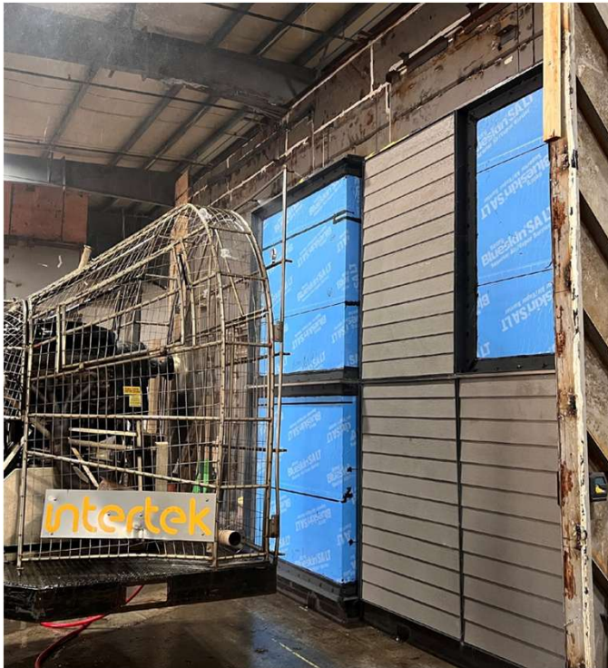
Performance Mock-Up Testing (AAMA 501.1)
