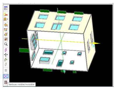
To create a component in WUFI Passive, in this case a floor, select the vertices in a counter-clockwise fashion, clicking each vertice while holding the CTRL key.
