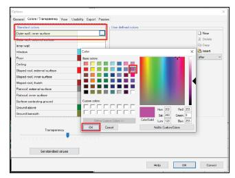
With the new color assigned, it becomes clear very quickly that the wall outlined in red is not oriented correctly and the newly assigned magenta inner side is facing outwards.
