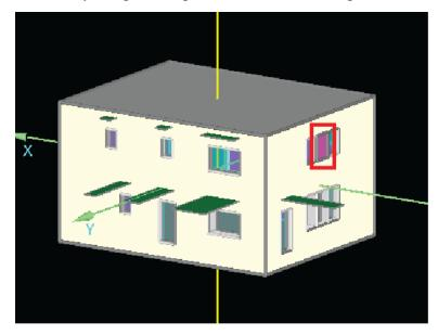
The most common components to be oriented incorrectly are windows. Windows are transparent and are assigned the same color on both the interior and exterior side, so it can be tricky to confirm the windows are oriented properly at first glance.
