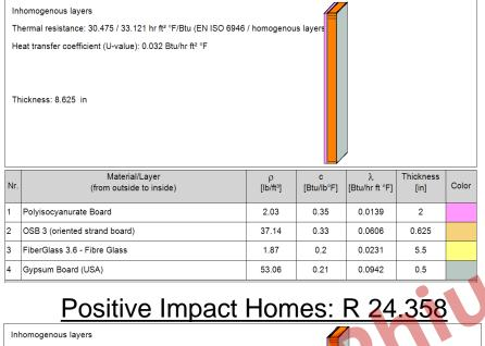
Thermal resistance: 24.358 / 27.111 hr ft² °F/Btu (EN ISO 6946 / homogenous layers Heat transfer coefficient (U-value): 0.039 Btu/hr ft² °F Thickness: 7.625 in
