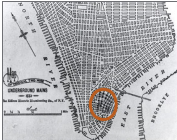
Fig. 1. Extent of the First Electric Grid in the US, essentially a Microgrid. 1
