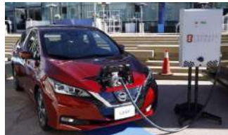
Figure 13: Nissan unveils the U.S. commercial offering of Vehicle to Home charging in Los Angeles for 2019 deployment in the U.S., using battery-powered Leaf cars and Fermata Energy bi-directional charging. 68
