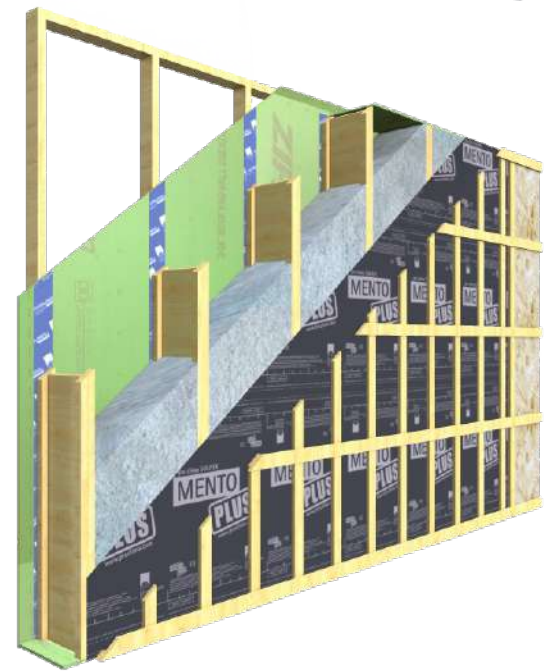
Above: wall section of Edgewaterhaus, Green design Studio, Double stud wall with air barrier on INTERIOR Right: Ecocor, prefabricated I-JOIST wall system.
