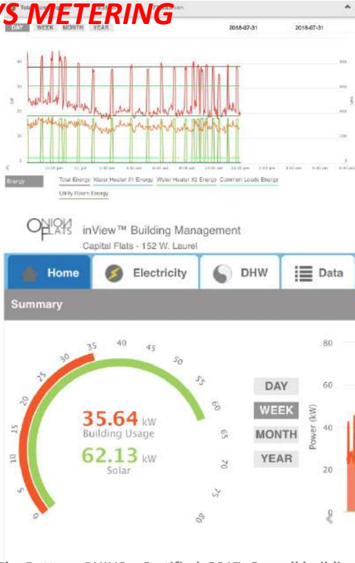
The Battery, PHIUS + Certified, 2017; Overall building consumption and electricity production
