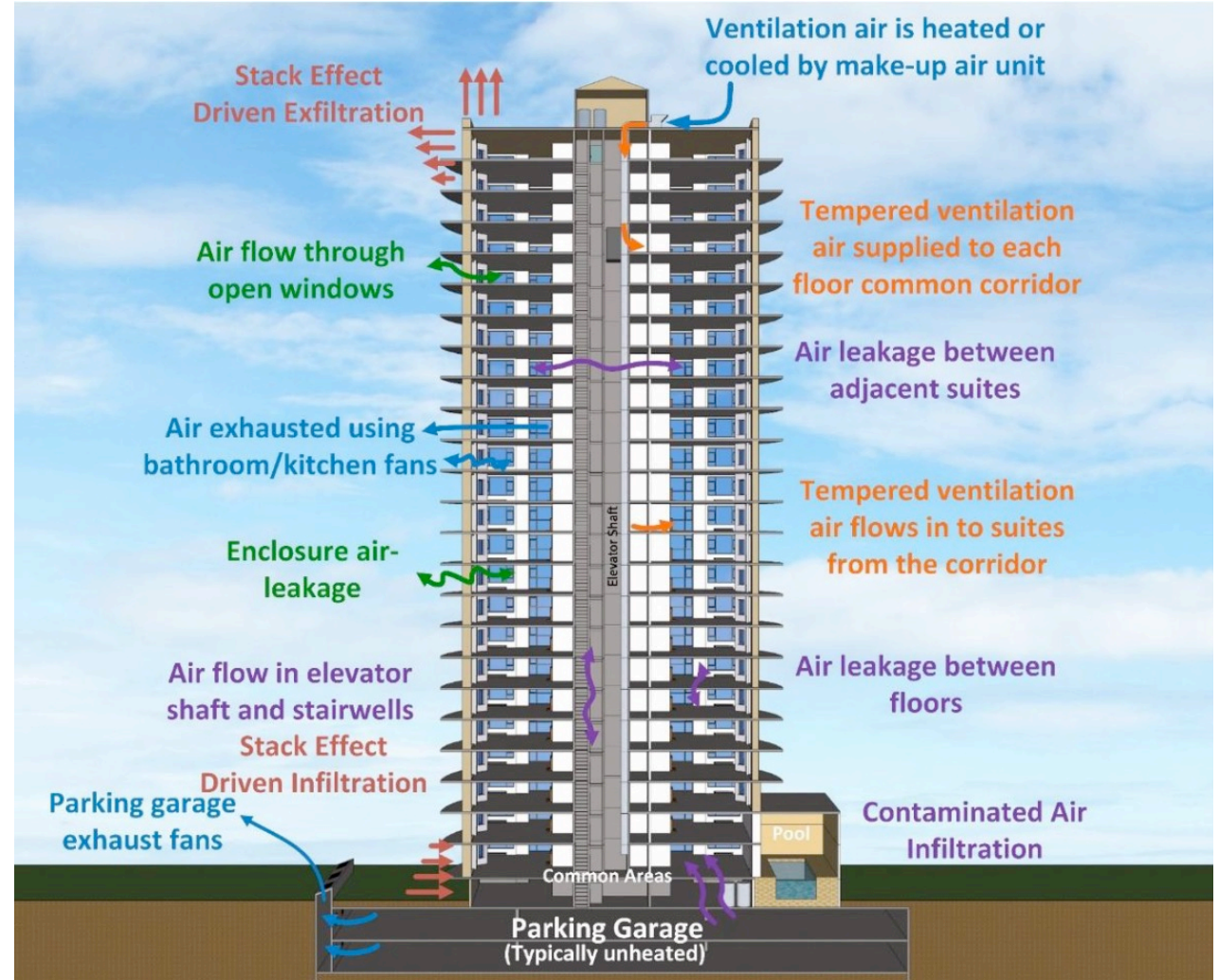
Typical Ventilation Approach in High-Rise MURBs 1
